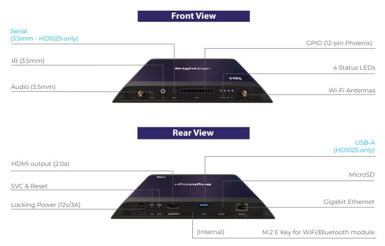
• USB Type A port: provides 5V/1A power to peripheral devices, such as touch screens
